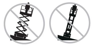
Do not raise the platform unless the machine is on a firm, level surface.
